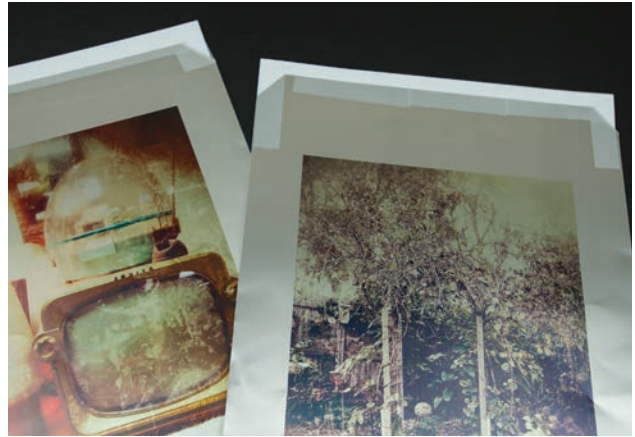
Printed blank offset plates showing leader paper attached.
